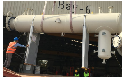
LL/H coalescer filter for water removal from ULSD (Ultra Low Sulphur Diesel).
