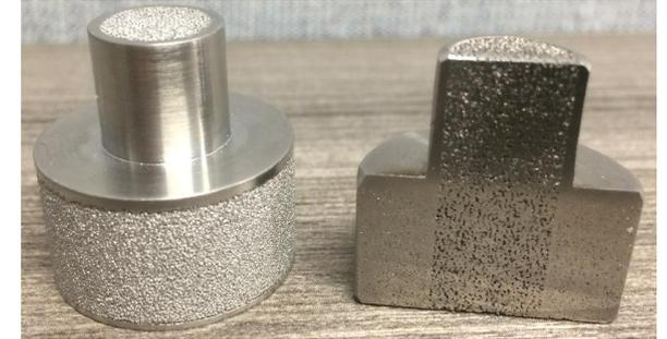
Example multi-dense porous used for thermal management application
