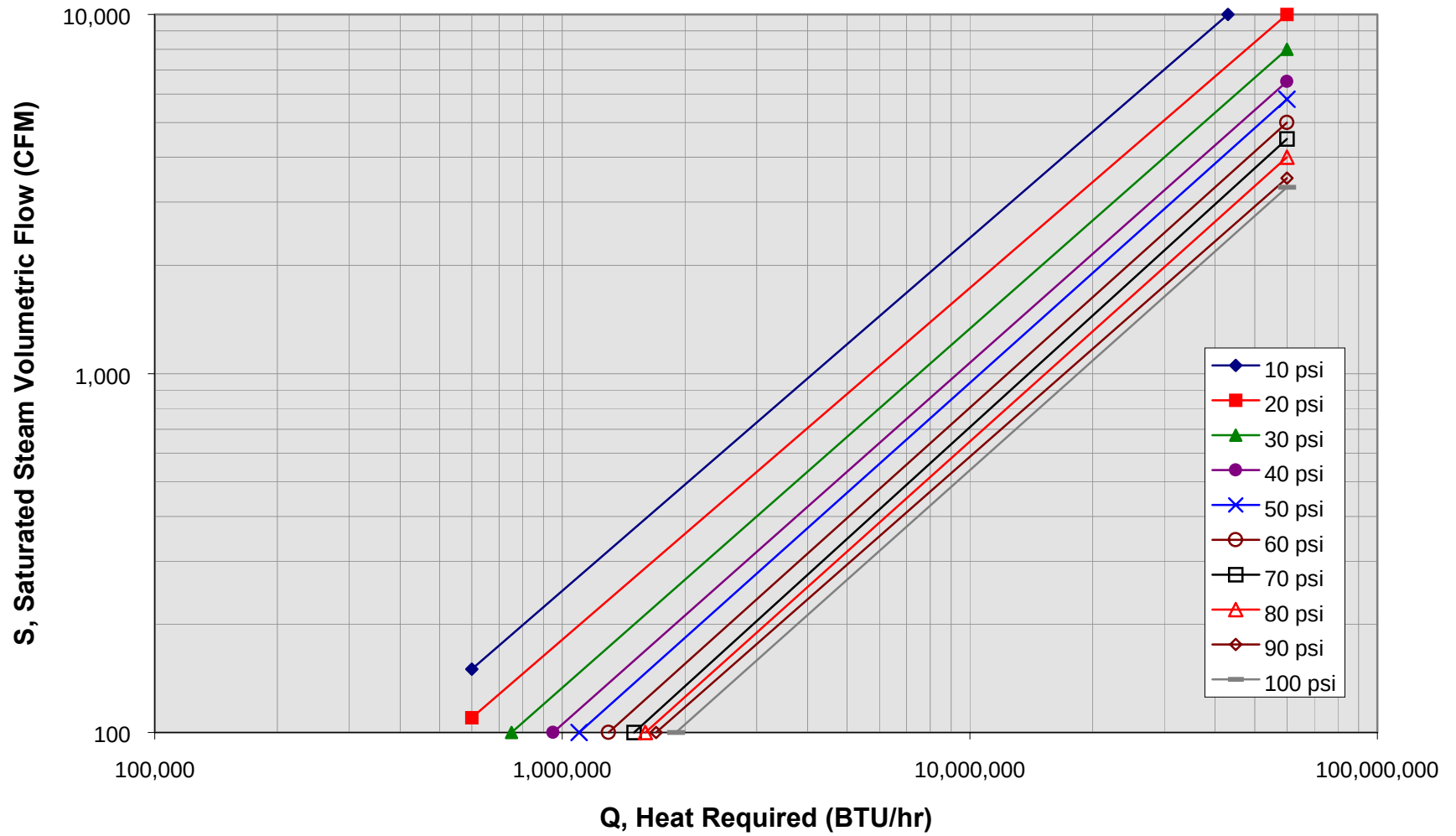
Figure 1: Heat Required vs. Saturated Steam Flow Rate
