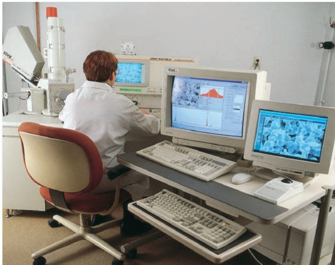
Among Mott's research and development assets is a scanning electron microscope (SEM), which enables Mott engineers to evaluate the physical properties of Mott media – right down to the size and shape of every pore.
