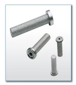
Series 6610 line filters are designed for line mounting in tubing with compression-type fittings. They are ideal for filtering liquids and gases to protect sensitive instruments.
