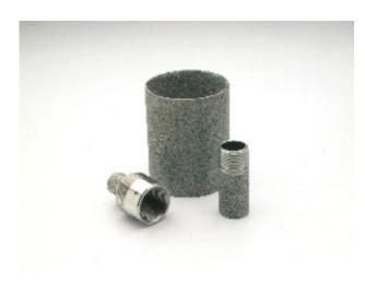
Flame Arrestors are safety devices that allow flow of combustible gases while preventing ignition. The Flame Arrestor prevents the flame from transferring to a different area of a device by cooling or quenching a flame front or by dampening a combustion wave. It is designed to absorb and dissipate the heat of a flame for specific operating and flow conditions. Integrating Mott's sintered metal media provides high strength and durability allowing these critical devices to perform precisely.
