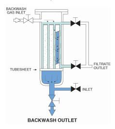
HyPulse LSM filters incorporate inside-out filtration within a double open-ended design. High-density solids are allowed to settle at the bottom of the filter vessel. LSM filters may be operated on a filter/ backwash cycle schedule, or can be used as concentrators in a recirculating system.
